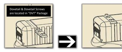
Step 3: Test fit the Red Dot sight to Outerimpact adapter, utilizing adjacent chart. Note: Make sure screws do not stick out beyond bottom of adapter. After test fitting, remove Red Dot sight from adapter.
