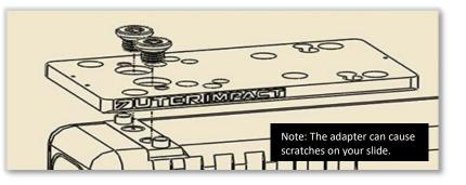
Note: The adapter has an intentional curve. This curve will flatten out when mounted.
